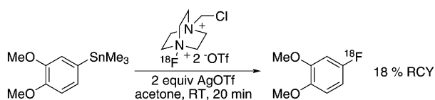
Scheme 15. 18 F Fluorodestannylation with [ 18 F]Selectfluor bis(triflate).
